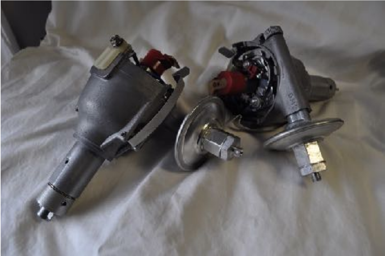
The distributors after rebuild
