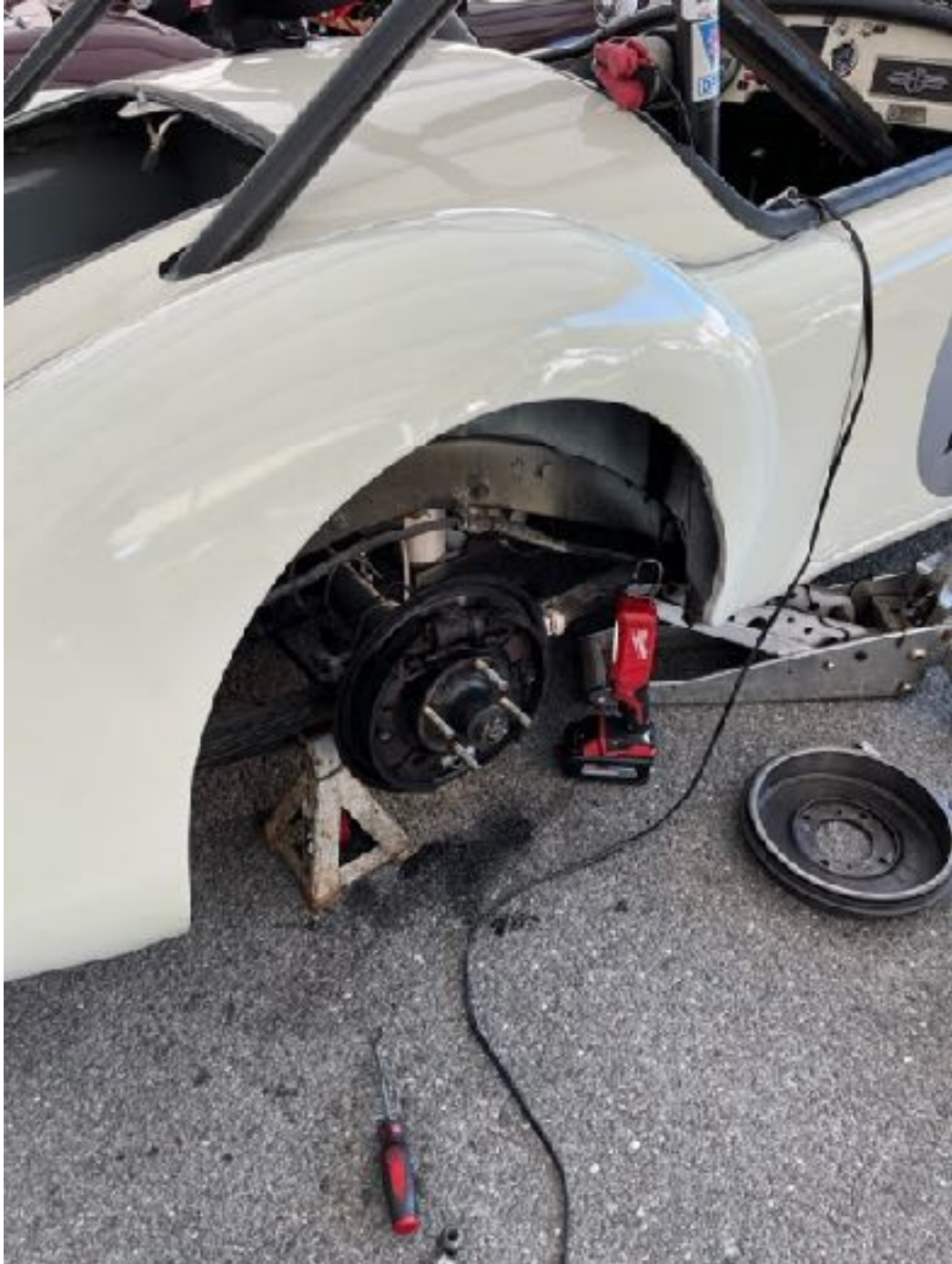
Axle seal failure
