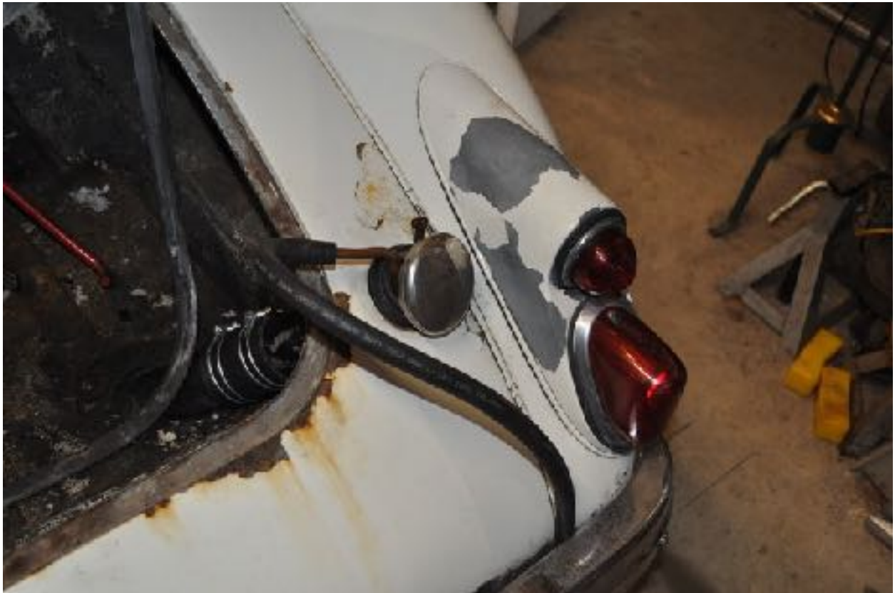
The temporary fuel feed fix
